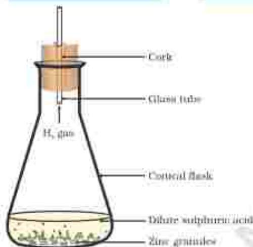
Figure 1.2 Formation of hydrogen gas by the action of dilute sulphuric acid on zinc
