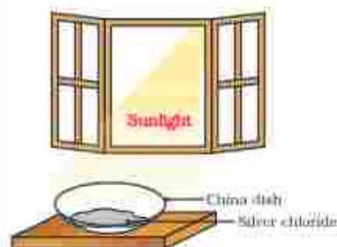
Figure 1.7 Silver chloride turns grey in sunlight to form silver metal
